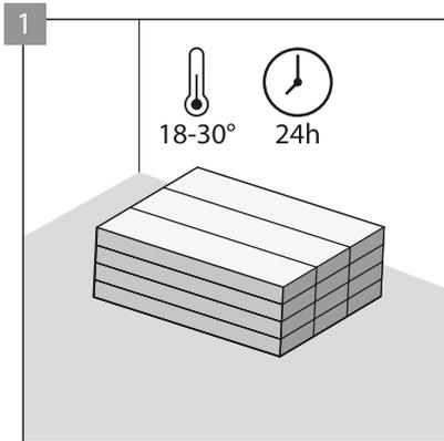
The installation mat should be stored at a temperature ranging between 5°C and maximum 35°C. Before the installation it should be subjected to the 48-hour acclimatisation at the temperature of 18-30°C, in the premises where it will be installed.
