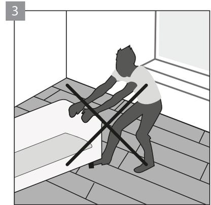
Directly after the installation, the floor may be walked upon gently, and heavy objects may be placed on the installed floor after 2 hours from the installation. The maximum adhesive strength is obtained after 24 hours following the installation; until that time, it is not recommended to move around any heavy objects or clean the floor.
